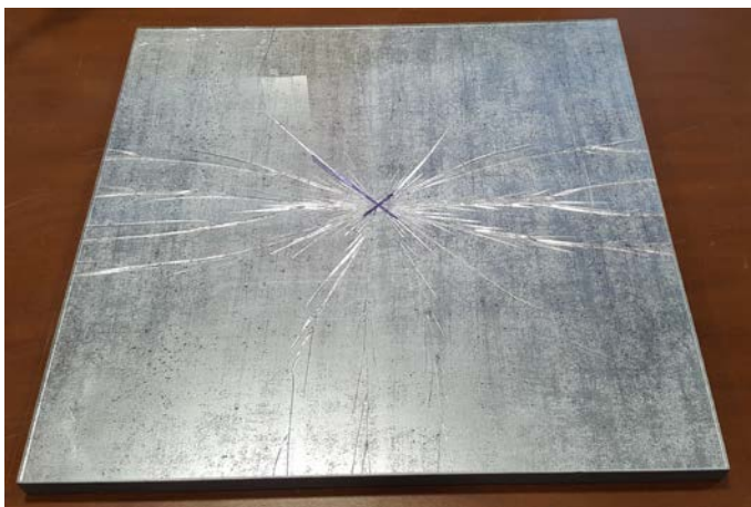
Figure 3. Example of tile fracture (centre and half side tests)
