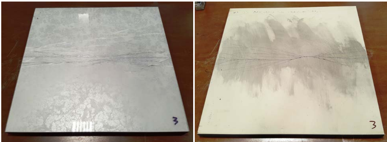
Figure 3. Example of tile fracture (front and back sides)
